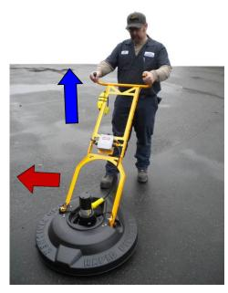
LIFT the handle and the machine will move to the RIGHT. NOTE: use moderate movements.
