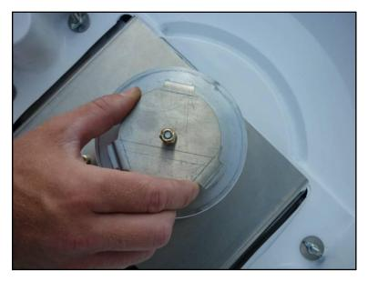
First, make sure the "legs" on the Cartridge Lock are aligned with the three protrusions on the Aluminum Clutch
