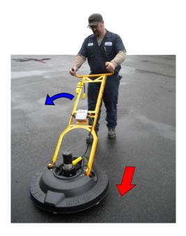
TWIST THE HANDLE TO THE RIGHT and the machine will move FORWARDS.
