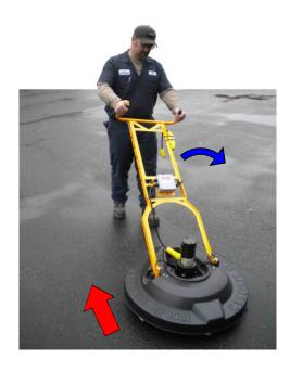
TWIST THE HANDLE TO THE LEFT and the machine will move BACKWARDS.
