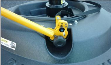
By using both the upper and lower holes for the Ball Lock Pins the handle angle can be adjusted in 5° increments
