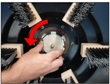
Rotate the Cartridge Lock counterclockwise to lock the Cartridge onto the Clutch.
