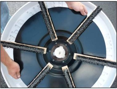
Place the Brush Cartridge onto the Aluminum Clutch
