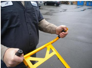
Make sure you are holding both handles securely before pushing the throttle button.
