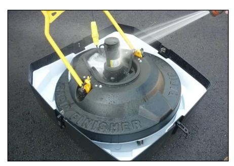
The motor can be washed with standard hose pressure. CAUTION: ALWAYS UNPLUG THE MACHINE FROM THE GENERATOR FIRST. Never use a pressure washer
