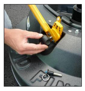
use the Ball Lock Pins to select the desired handle height
