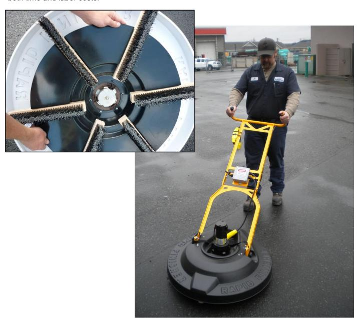
This fast and easy machine works in a similar manner to a floor polisher, with a multi-brush Cartridge that effortlessly works the coatings into the asphalt surface at variable speeds up to 70 rpm. Each brush Cartridge has a usable life of 5,000 ft<sup>2</sup> (500 m<sup>2</sup>) or more, and the brushes are easily replaceable.
