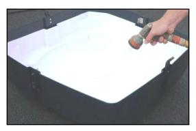
If the Liners need to be replaced a liner kit (part number 80-0-403A), that contains 2 Base Liners and 2 Case Liners, is available from Integrated Paving Concepts. The Base Liner is secured by 4 wing nuts and large washers on the underside.
