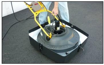
Lower the machine into the water and run the brushes at a slow speed until the brushes are clean
