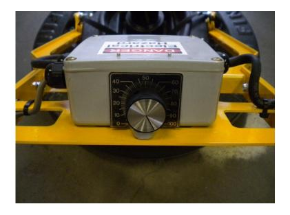
To adjust the rotation speed of the brushes simply adjust the dial on the control box.
