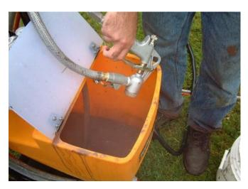
Cycle the water through the system making sure that both the gun hose and the recycle hose are thoroughly flushed of coating.
