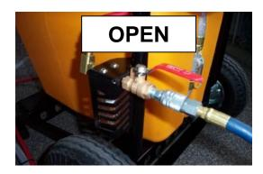
With compressor running, open the air valve to start the pump. Coating should begin to recirculate, with the pump "ticking" over at a slow rate.
