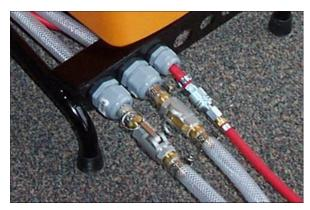
Connect the recirculation hose, discharge hose and air hose to the hopper and pump as shown
