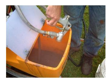
To attain the optimum spray pattern spray back into the hopper while adjusting air pressure and material flow on the gun.
