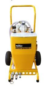
**Power Requirements**: The air supply is from a compressor (not supplied) which is capable of supplying at least 12-14 cfm (0.3 cubic meters/ min.) of continuous air at 60-80 psi. (400-550 atmospheres).
