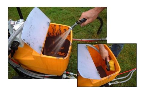
When finished using sprayer and gun, pump remaining coating into bucket and turn off pump. Pour clean water into hopper and clean with supplied yellow gong brush to remove as much coating as possible.
