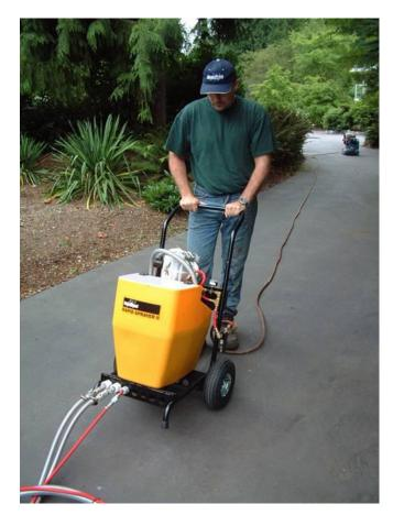
Place the compressor at the finish point of the job as shown to best keep the hoses out of the way.
