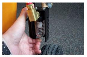
Make sure the air filter has been purged of water. To drain, press button on underside as shown.
