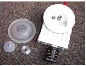
Use a 7/8" wrench and socket to remove the diaphragm from the shaft and piston. Use a vise (with protective jaws to prevent any damage to the shaft) to remove the diaphragm from the other side.
