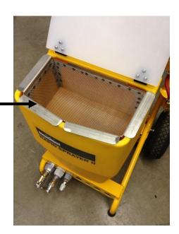
Recommended Maximum fill line. The hopper will hold more coating than this (10 gallons), but the unit is more difficult to move around the job site.
