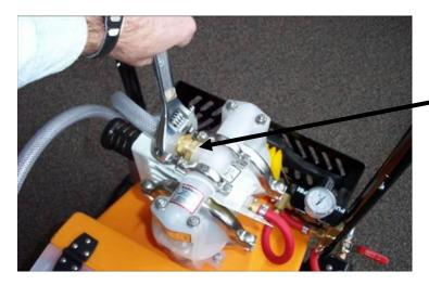
Detach the discharge hose on the top of the pump (this is a regular garden hose fitting)
