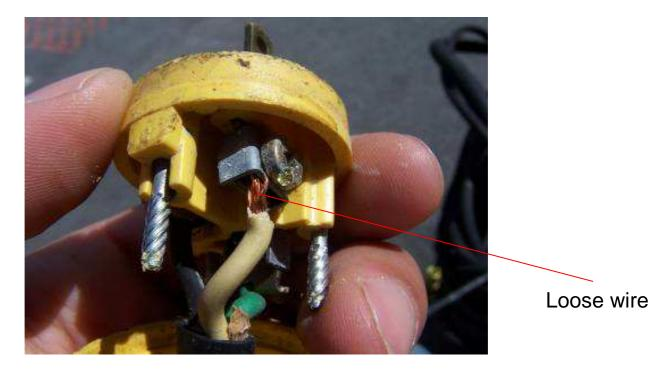
2. Remove sleeve and tighten / re-wire any loose wires.
