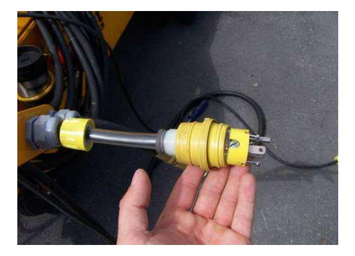
Before checking for loose wires, make sure all connections are un-plugged and are not live.
