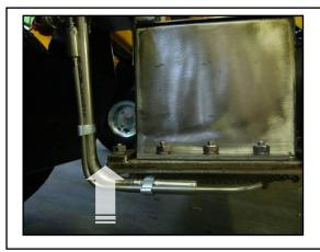
5c. When re-installing the pilot lights, make sure they are **positioned as close as possible to the underside of the heaters** so that they are less vulnerable to being damaged.
