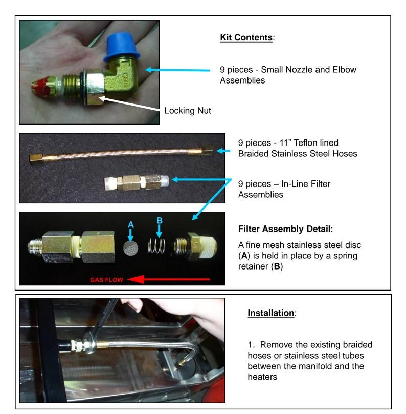
2. Note: It is easier to replace the Nozzle assemblies if the wing heaters are removed from their frame. The center heaters can remain attached.
