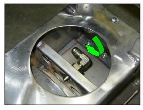
4. Unscrew the whole assembly from the mounting bracket. Replace with the Small Nozzle Assemblies and tighten the locking nut.
