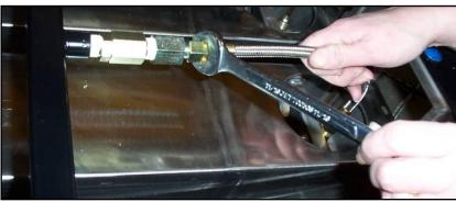
10. Then attach the other end of the hose to the Filter Assembly. VERY IMPORTANT: Use Compressed air and soapy water to check for leaks. Reseat and tighten fittings if necessary.
