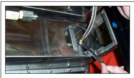
9. Install the new (shorter) 11" Braided Hoses. Start by installing and tightening the hose onto the Heater Nozzle assembly as shown
