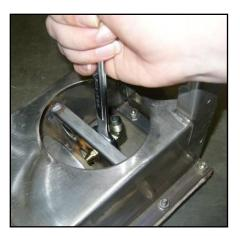
3. Use an 11/16" wrench to loosen the locking nut on the large nozzle assembly installed in the heater.
